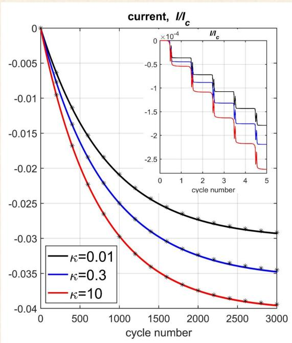
Solid lines - numerical solution of the thin shell model + circuit eq. for the coil; black stars "\*" - analytical solutions for the simplified model.
