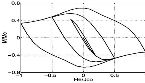
**FIG. 9.** Hysteresis loops (Kim model). Normalized magnetic moment  $M/M_0$  against external magnetic field,  $M_0 = |\Omega|J_{c0}/4$ .
