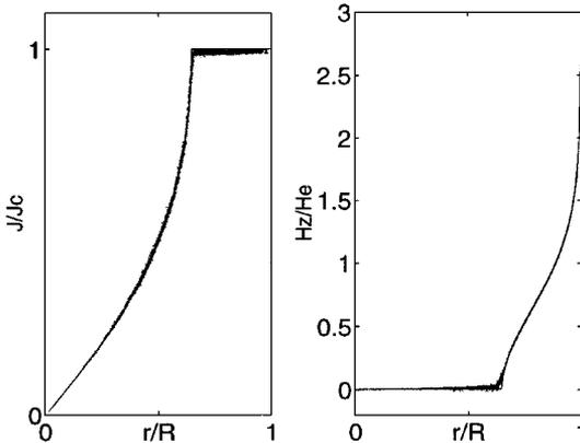
**FIG. 2.** The analytical and numerical solutions for a thin disk: the current density (left) and normal component of magnetic field (right). The values of  $J$  and  $H_z$  in each finite element are plotted against the radial coordinate of the element center as distinct points. These points are close to the solid lines representing the analytical solutions. The external field is  $H_c/J_c = 0.5$ . The finite element mesh contained 3416 nodes and 6670 elements.
