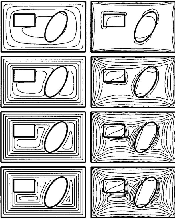
**FIG. 7.** Magnetization of a multiply connected film. The current contours (left) and level contours of magnetic field (right). The external magnetic field  $H_e/J_c = 0.25, 0.50, 0.75, 1$ .
