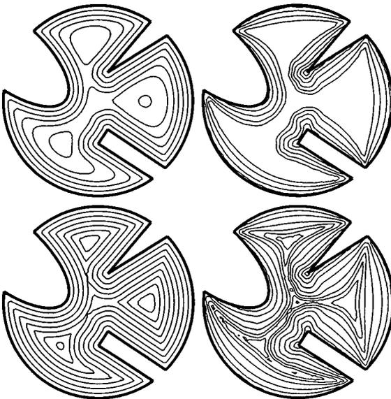
**FIG. 4.** Magnetization of an irregularly shaped film. The current contours (left) and level contours of magnetic field (right). The external magnetic field  $H_e/J_c = 0.5, 1$ .
