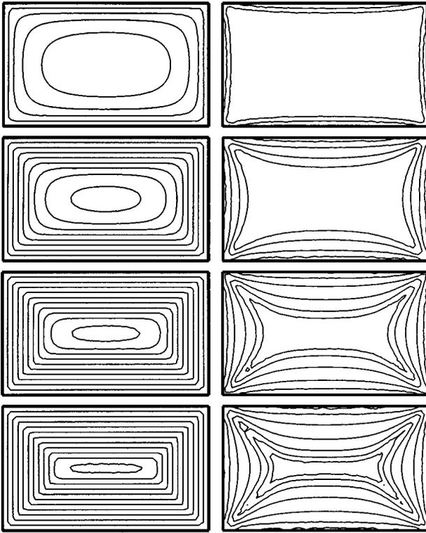
**FIG. 3.** Magnetization of rectangular film. The current contours (left) and the level contours of magnetic field at the film midplane (right). The external magnetic field  $H_e/J_c$  (from top to bottom): 0.25, 0.50, 0.75, 1. Finite element mesh: 1424 nodes, 2728 elements.
