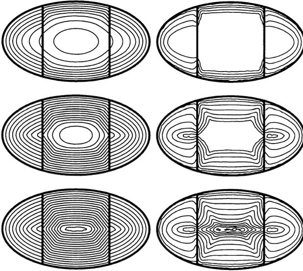
**FIG. 5.** Magnetization of an inhomogeneous film. The current contours (left) and level contours of magnetic field (right). The critical current density:  $J_c$  in the left and right parts,  $1.5J_c$  in the middle part of the film. The external magnetic field  $H_e/J_c = 0.5, 1, 1.5$ .
