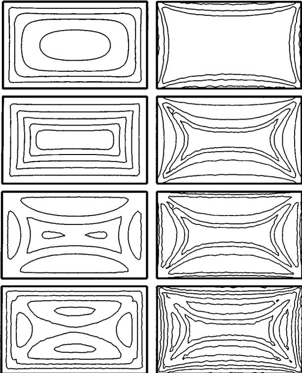
**FIG. 8.** Magnetization of a film in a non-monotone external field (Kim model). The critical current density:  $J_c = J_{c0}/(1 + |H_z|/H_0)$ , where  $H_0/J_{c0} = 0.5$ . The external magnetic field:  $H_e/J_{c0} = 0.25, 0.50, 0.25, 0$ .
